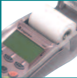
"Easy load" 15 lines per second thermal printer
